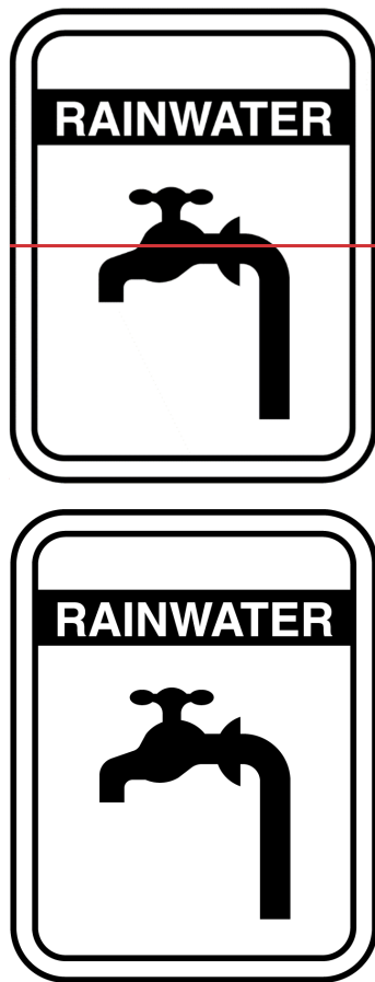
Figure 15.3.2.24 — Typical sign for rainwater outlets outlet
